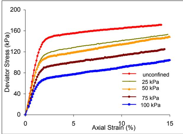
Figure 9. Stress-Strain Curves for EPS26 (Duration of Confinement = 24 hrs.)
