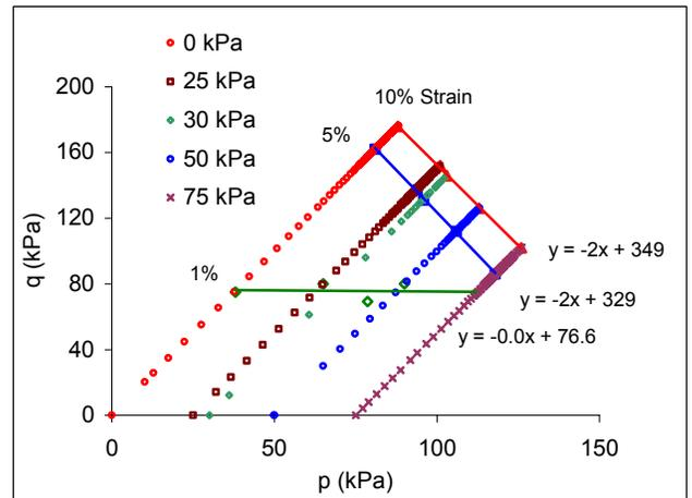
Figure 12. Stress Path for EPS26 During Triaxial Compression
