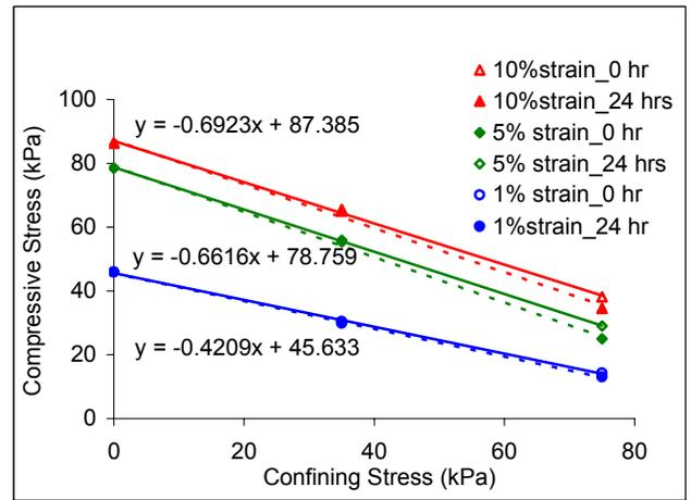
Figure 6. Strength of EPS16 with Confining Stress and Duration of Confinement
