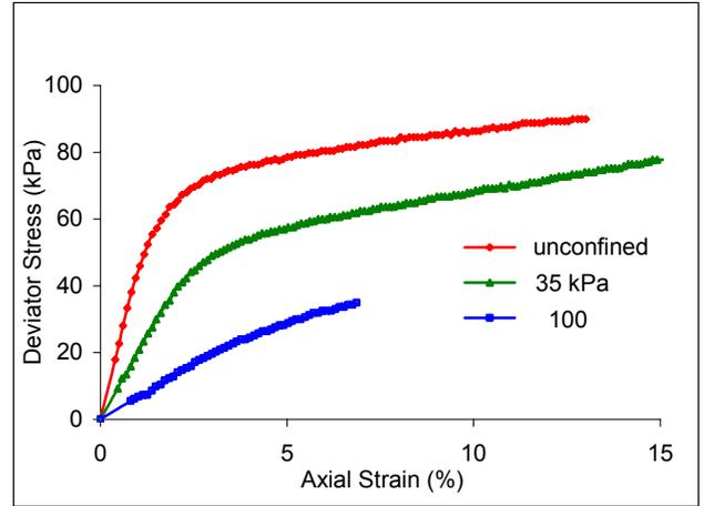
Figure 4. Stress-Strain Curves for EPS16 (Duration of Confinement = 3 hrs.)
