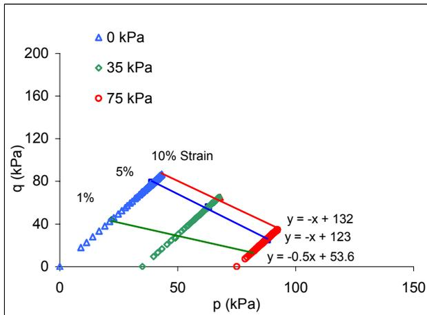
Figure 11. Stress Path for EPS16 During Triaxial Compression
