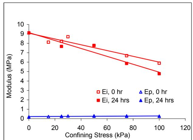
Figure 14. Modulus of EPS26 with Confining Stress (Duration of Confinement = 0 and 24 hrs.)
