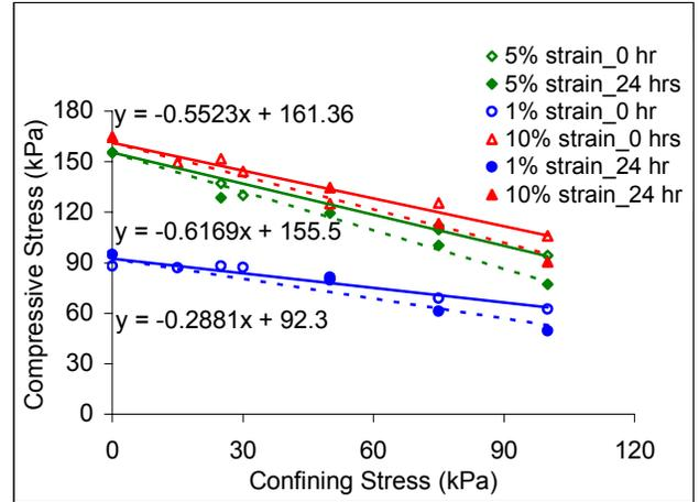
Figure 10. Strength of EPS26 with Confining Stress and duration of confinement
