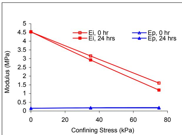
Figure 13. Modulus of EPS16 with Confining Stress (Duration of Confinement = 0 and 24 hrs.)
