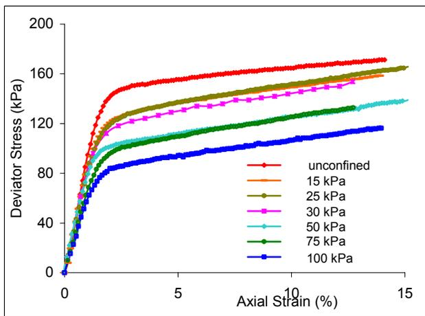
Figure 7. Stress-Strain Curves for EPS26 (Duration of Confinement = 0 hr.)
