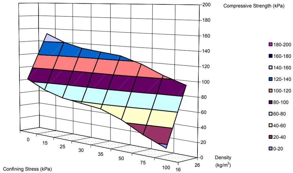
Figure 18. Compressive Strength at 5% Axial Strain
