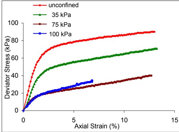
Figure 3. Stress-Strain Curves for EPS16 (Duration of Confinement = 0 hr.)
