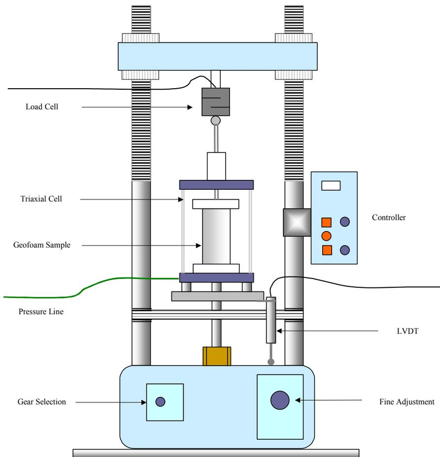
Figure 2. Diagram of Triaxial Test Setup
