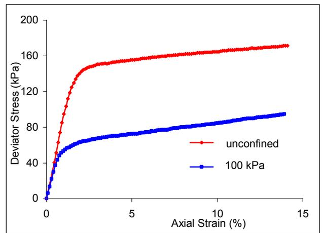
Figure 8. Stress-Strain Curves for EPS26 (Duration of Confinement = 3 hrs.)
