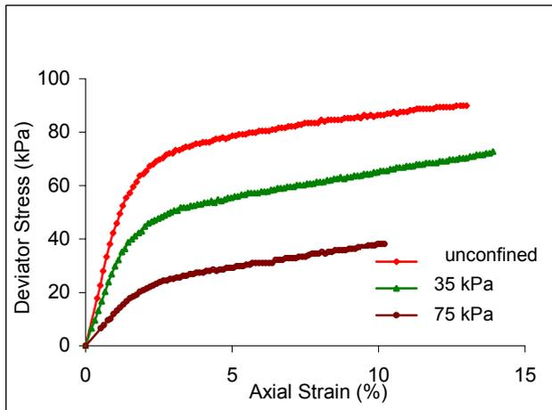
Figure 5. Stress-Strain Curves for EPS16 (Duration of Confinement = 24 hrs.)
