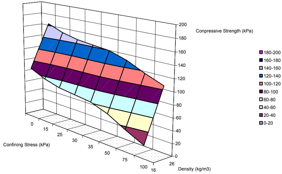
**Figure 19. Compressive Strength at 10% Axial Strain**
