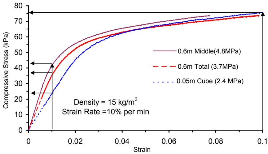
Figure 1. Effect of Sample Size on Compressive Strength (After Elragi, 2000)
